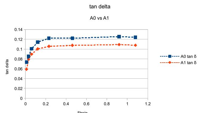
The above comparison of tan delta of the two vulcanizates cured to Tc90 demonstrates the dynamic property improvement capability with DPG elimination.
