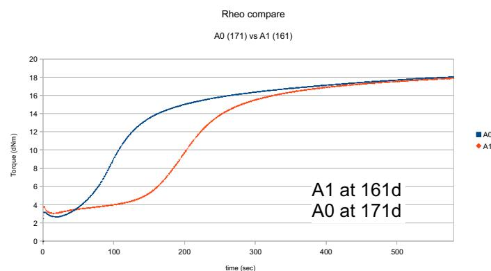
The cure time was chosen to be 9.72 min for both the A0 (DPG control) and the A1 (DPG free with 2phr Premix Acti8). It is apparent that the rheometry is the same shape and cure profile at and after the cure time. Note that this is done with a 10 deg reduction in cure temperature on the A1 material.
